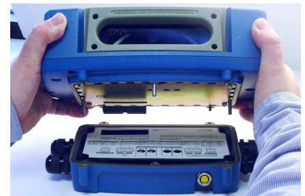
Installing Scan Head to Wiring Base
